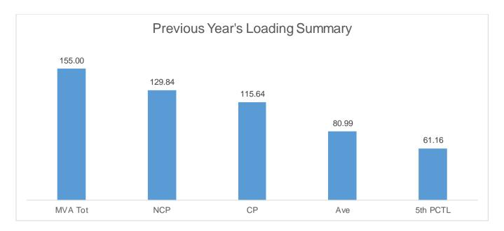
The Non-coincident Peak Demand is 129.84 MW, which is around 83.77% of the total substation capacity of 155 MVA at a power factor of 0.98. The load factor or the ratio between the Average Load of 80.99 MW and the Non-coincident peak demand is 62.37%. A safe estimate of the true minimum load is the fifth percentile load of 61.16% MW which is 47.10% of the Non-coincident Peak demand.
