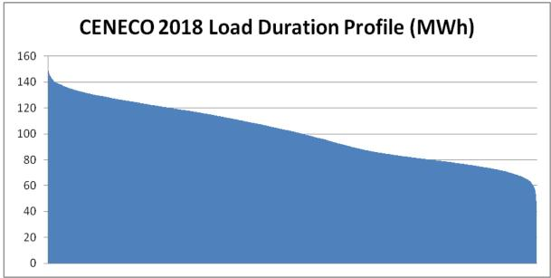
CENECO 2018 annual load profile depicts a baseload of 71 MW with a load factor of 99.47%, a mid-merit load of 48 MW with a load factor of 58.13% and a peaking load of 30 MW with 7.92% load factor.
